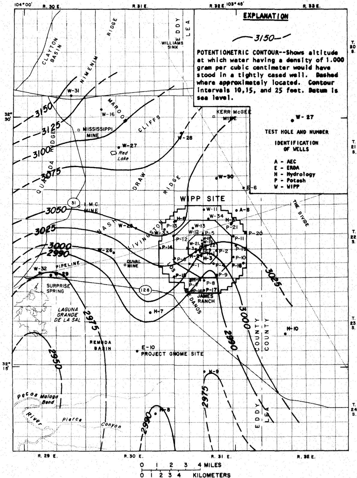
Figure 17.--Adjusted potentiometric surface of the Culebra Dolomite Member of the Rustler Formation (1982) at and near the proposed Waste Isolation Pilot Plant (WIPP) site.
