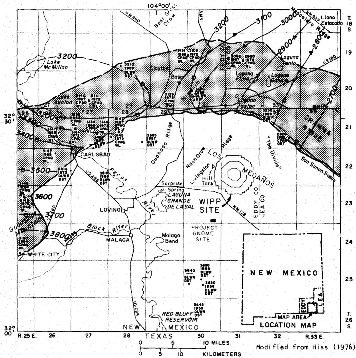
Figure 11.--Potentiometric surface of the Capitan aquifer in the vicinity of the proposed Waste Isolation Pilot Plant (WIPP) site.
