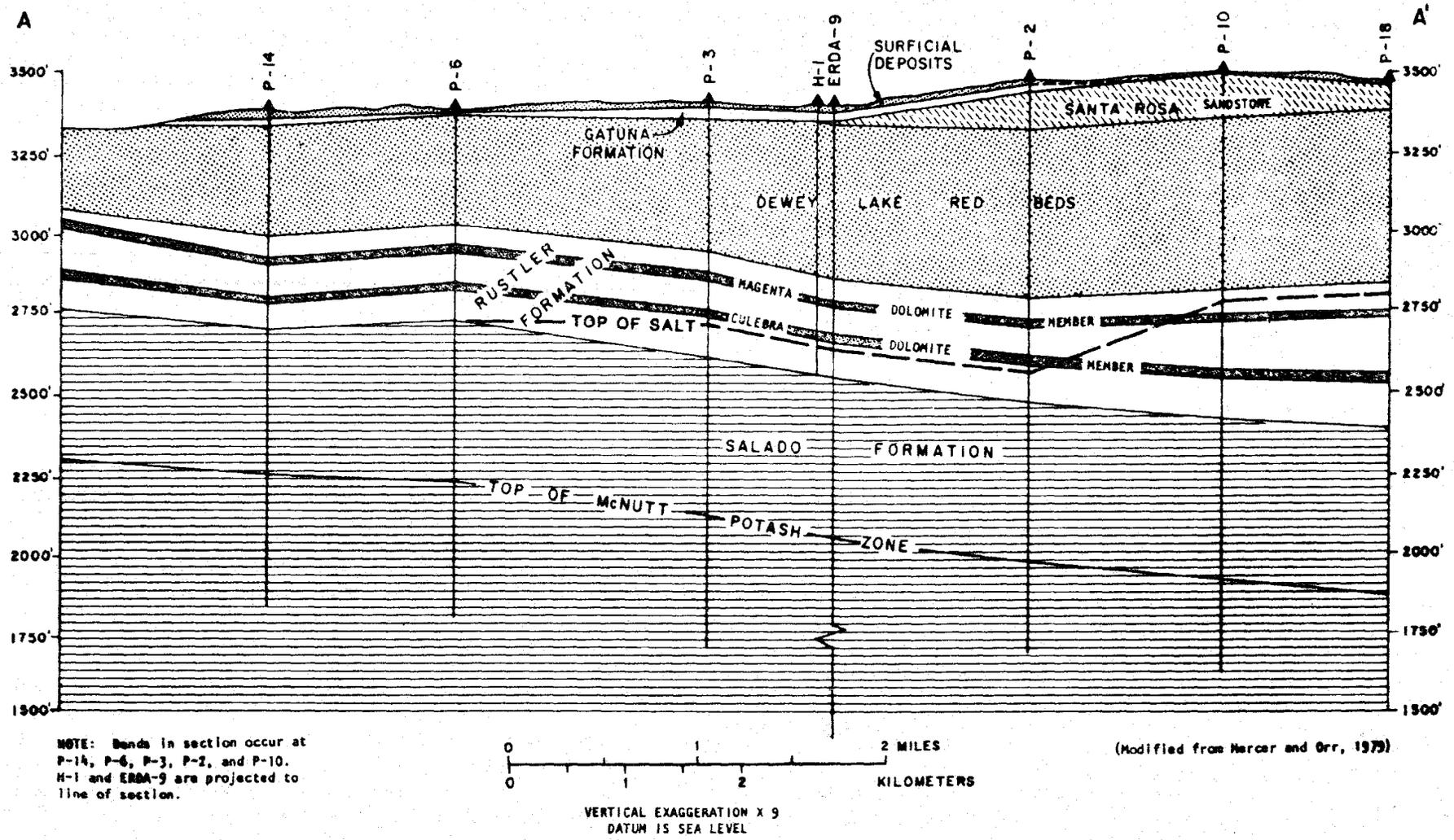
Figure 5.--Geologic section across the proposed Waste Isolation Pilot Plant (WIPP) site.
